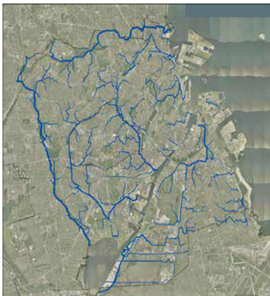
Copenhagen Flow Routes/ Areas with highest risk of significant damage as a result of high-intensity rainfall
