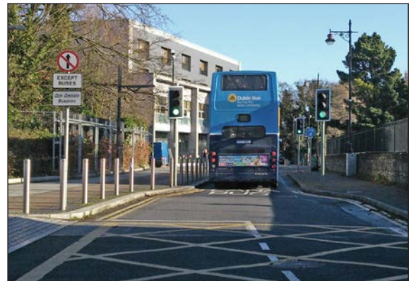
Figure 3.29: Example of a 'bus gate' in Tallaght, Co. Dublin, which filters permeability to allow for the free passage of buses whilst excluding other vehicles.
