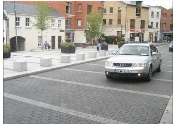
Figure 4.57: Example from Chapelizod, Co. Dublin, where the carriageway has been paved adjacent to a square in a village centre to add value to place and calm traffic in an area of higher pedestrian activity.
