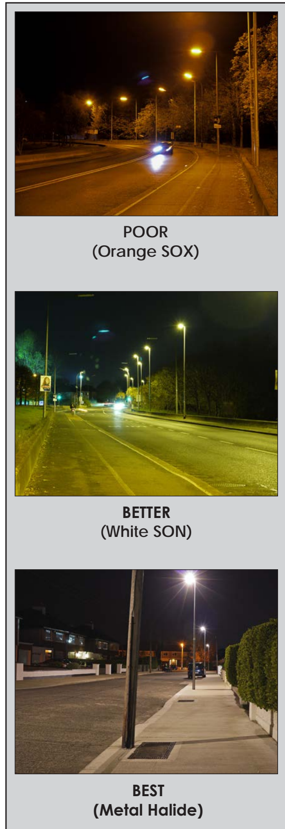
Figure 4.21: Examples of differing types of lighting and their effectiveness in terms of safety and placemaking.
