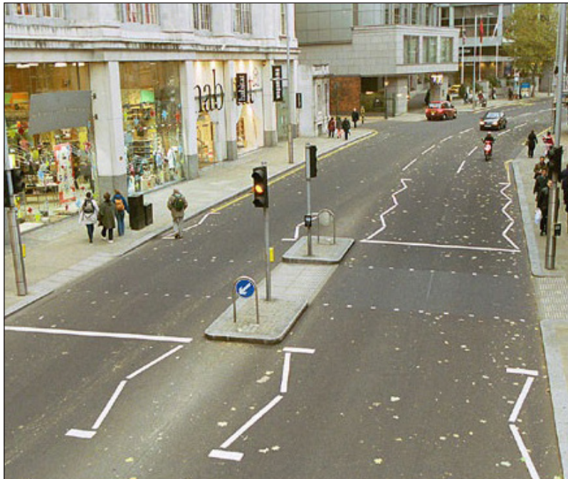
Figure 4.16. Kensington High Street, London, UK, where as part of upgrade works, a major decluttering exercise took place which included removing all guardrails, minimising signage and line marking. It is notable that upon completion of the works, vehicle speeds decreased and the incidence of accidents decreased by 43% (2003-2005). Left image source: Kensington and Chelsea Borough Council.
