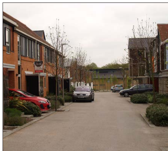
Figure 4.79. Example from New Hall, UK where a variety of in-curtilage and on-street parking is provided. On-street parking is provided semi-informally (indicated by the planting of trees). The parking of vehicles further calms traffic by providing a series of horizontal deflections.
