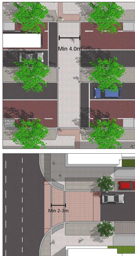
Figure 4.41: Standard crossing widths to be used in most circumstances across the main carriageway of Access or Link streets and across side junctions with Local streets.
