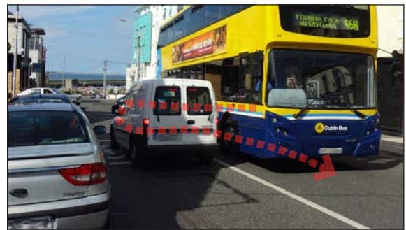
Figure 4.45: Setback stop lines allow for additional vehicular manoeuvrability for larger vehicles at signalised junctions without the need for larger corner radii.
