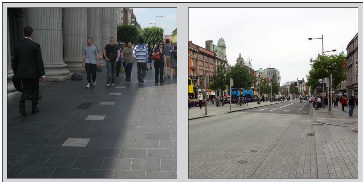
Figure 4.23: O'Connell Street, Dublin. The high place status, intensity of activity and low design speed (30 Km/h) is highlighted by high quality and robust materials, such as granite paving.
