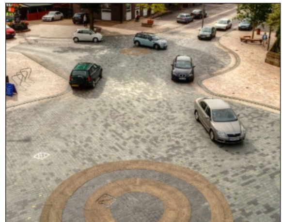
Figure 4.61: Examples from Ashford, UK (top) and Poynton, UK (bottom). The placement of a circular features with the shared space/traffic calmed environment creates an informal roundabout with fewer restrictions pedestrian/cyclist movement when compared to more conventional types (image sources: Hamilton-Baillie Associates and Ashford Borough Council).
