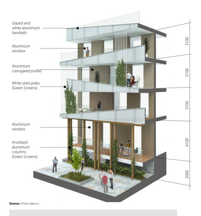
Diagram showing street level condition for ground floor units and balconies.
