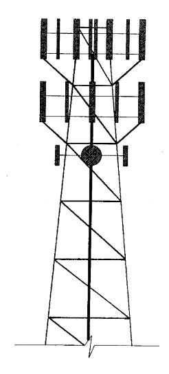
The visual impact of a shared structure should be carefully considered. In addition to the increased number of antennae the height, width and bulk of the structure and of the structural members will be increased. Cable trays to cater for at least 21 cables will be required.
