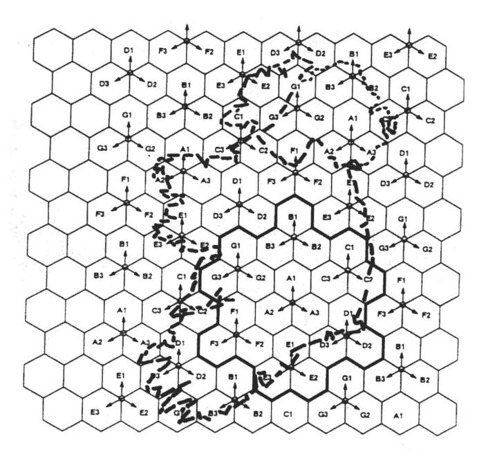
Division into cell pattern facilitates reuse of frequencies but never in adjoining cells. In reality cells are not regular in shape and they vary in size.
